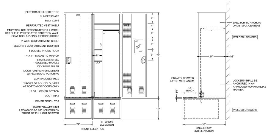
WELDED LAW ENFORCEMENT LOCKER FRAMES 24" X 24" X 72" S.R.S.T. W/ WELDED LOWER COMPARTMENT 24" X 36" X 18"
