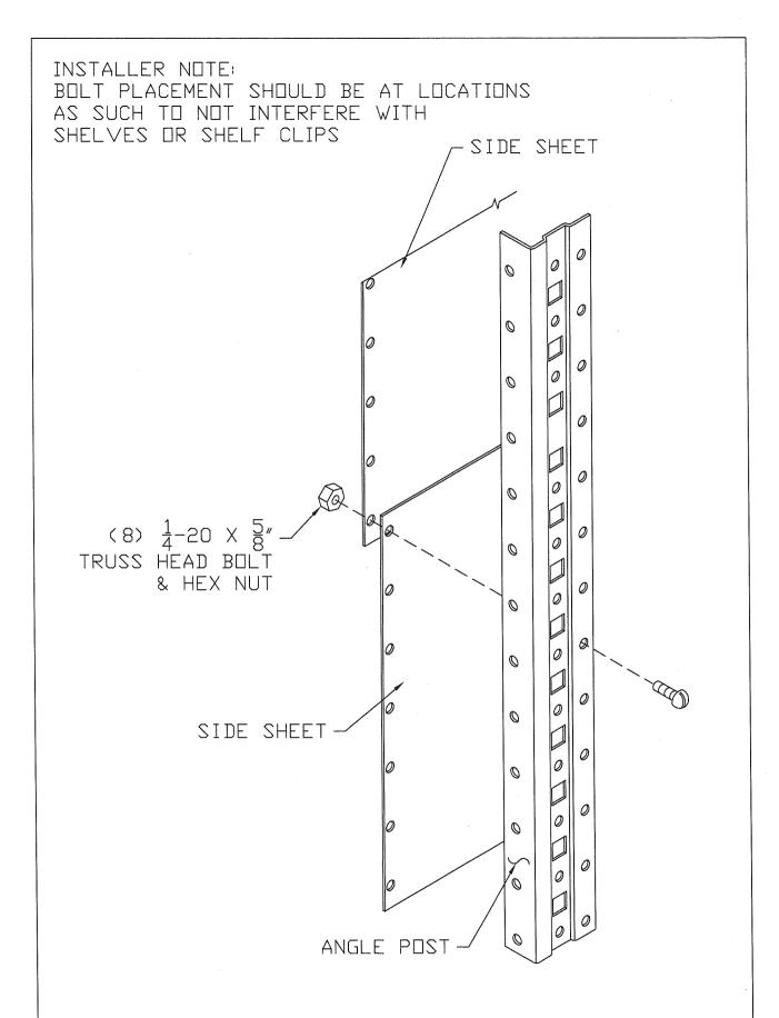
CONNECTION DETAIL SIDE SHEET WITH OVERLAP
