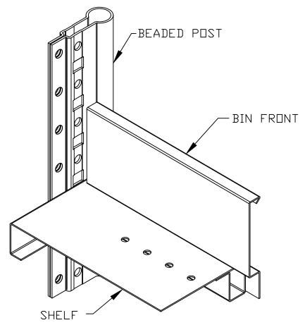
INSTALL BY POSITIONING BIN FRONT BEHIND THE FACE OF THE POST AS SHOWN ABOVE. TO FASTEN ALIGN BOTTOM OF THE BIN FRONT LIP WITH THE HOLES LOCATED IN THE FACE OF THE SHELF AND USE (3) PANEL CLIPS.
