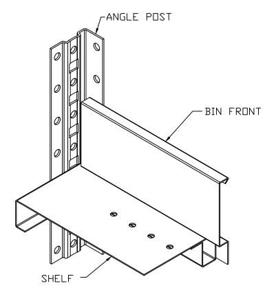
INSTALL BY POSITIONING BIN FRONT BEHIND THE FACE OF THE POST AS SHOWN ABOVE. TO FASTEN ALIGN BOTTOM OF THE BIN FRONT LIP WITH THE HOLES LOCATED IN THE FACE OF THE SHELF AND USE (3) PANEL CLIPS.
